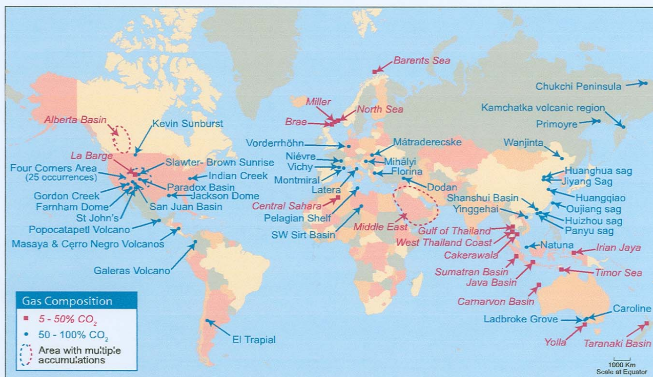
Figure 5.11 Examples of natural accumulations of CO 2 around the world. Regions containing many occurrences are enclosed by a dashed line. Natural accumulations can be useful as analogues for certain aspects of storage and for assessing the environmental impacts of leakage. Data quality is variable and the apparent absence of accumulations in South America, southern Africa and central and northern Asia is probably more a reflection of lack of data than a lack of CO 2 accumulations.
